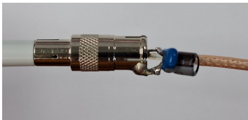
Figure 77 – Oscilloscope Probe with Cal Test CT2708 BNC Adapter. (Modified with Wires for Ripple Measurements, and a Parallel Decoupling Capacitor Added.)
