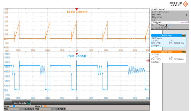
Figure 74 – 230 VAC, 42 V LED Load. Upper: I_{DRAIN} , 1 A / div. Lower: V_{DRAIN} , 100 V / div., 10 \mu s / div.
