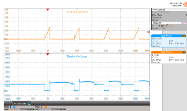
Figure 78 – 100 VAC, 42 V LED Load. Upper: I_{DRAIN} , 1 A / div. Lower: V_{DRAIN} , 100 V / div., 20 µs / div.
