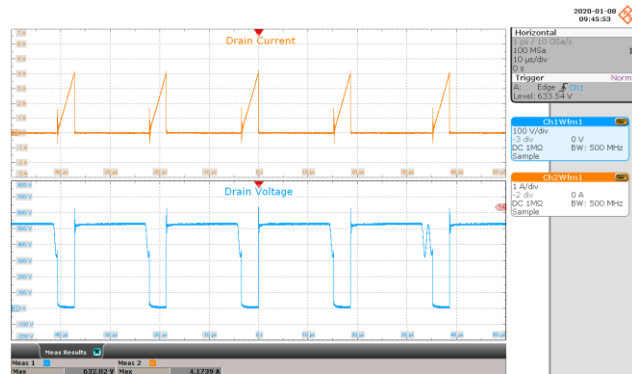
Figure 72 – 120 VAC, 42 V LED Load. Upper: I_{DRAIN} , 1 A / div. Lower: V_{DRAIN} , 100 V / div., 10 \mu s / div.
