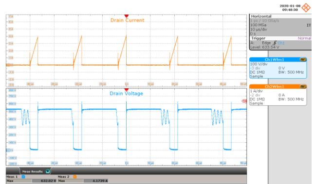
Figure 76 – 277 VAC, 42 V LED Load. Upper: I_{DRAIN} , 1 A / div. Lower: V_{DRAIN} , 100 V / div., 10 \mu s / div.
