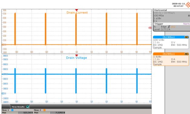
Figure 83 – 277 VAC, Output Shorted. Upper: I_{DRAIN} , 1 A / div. Lower: V_{DRAIN} , 100 V / div., 1 s / div.
