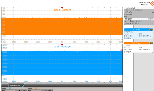
Figure 71 – 120 VAC, 42 V LED Load. Upper: I_{DRAIN} , 1 A / div. Lower: V_{DRAIN} , 100 V / div., 4 ms / div.
