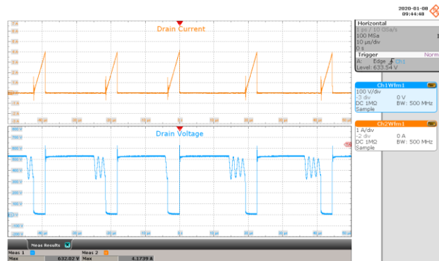
Figure 70 – 100 VAC, 42 V LED Load. Upper: I_{DRAIN} , 1 A / div. Lower: V_{DRAIN} , 100 V / div., 10 \mu s / div.
