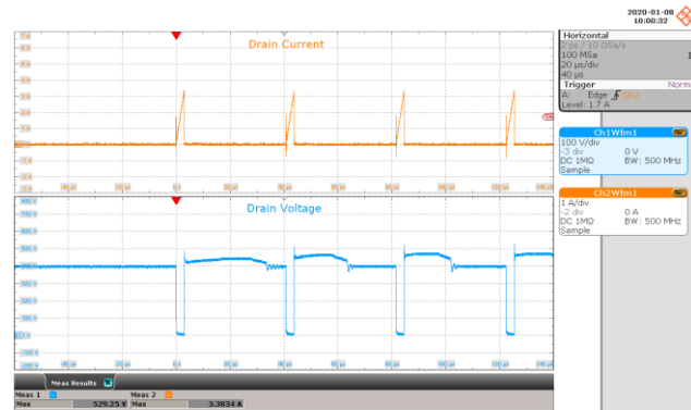
Figure 80 – 277 VAC, 42 V LED Load. Upper: I_{DRAIN} , 1 A / div. Lower: V_{DRAIN} , 100 V / div., 20 µs / div.
