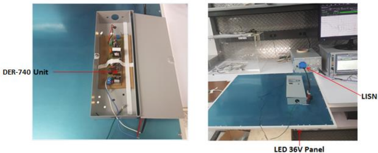
Figure 88 — Conducted EMI Test Set-up.
