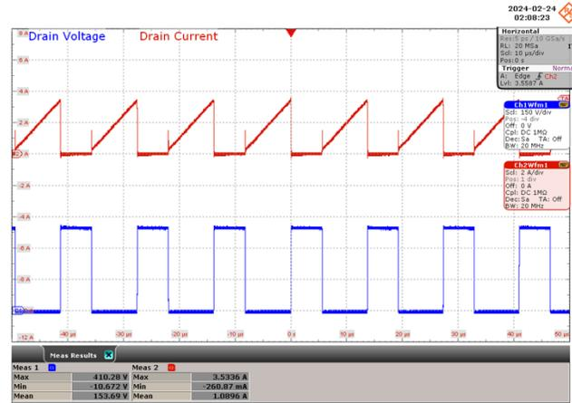
**Figure 59** – 120 VAC, 42 V LED Load.
