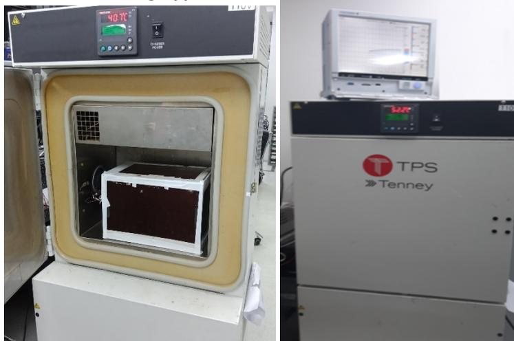
Figure 44 – Test Set-up Picture – Unit Inside Mechanical Casing.
